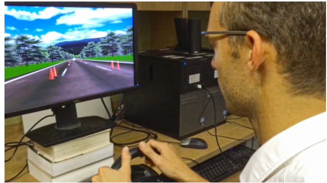
Figure 3. Physical setup – the participant's eye is fixed 50 cm away from the screen, providing a \sim 62^\circ horizontal viewing angle. Driving simulator is controlled with a racing wheel.
